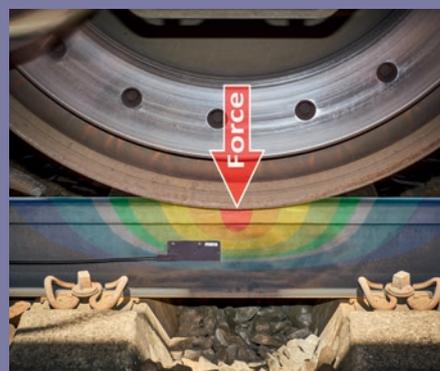
For the past 50 years, axle counting technology was based on electromagnetic sensors. Thales has developed a new generation of sensor, fibre optic based which will revolutionise axle counting, especially when it comes to investment and life-cycle cost:
