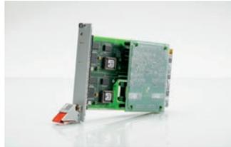
The serial board is the link between the indoor system and the detection point in the outdoor plant. It forwards the counter data of each detection point to the CPU.
